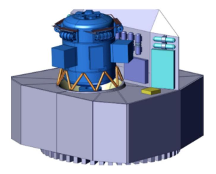
X-IFU mounted on the Science Instrument Module. Courtesy of M. Ayre (ESA study team). X-IFU dewar design is currently undergoing a final design iteration (not shown here)
