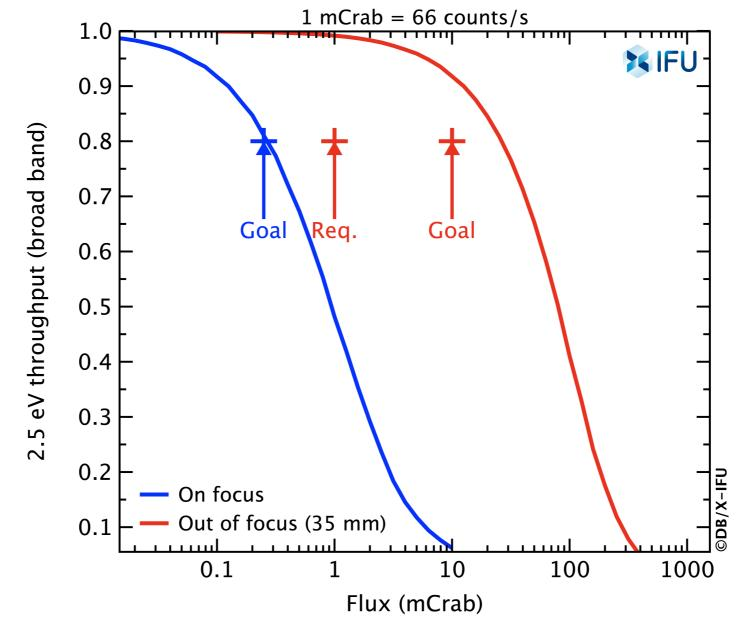
Count rate performance in different mirror and instrument configurations (Courtesy of Th. Dauser and E. Cucchetti)
